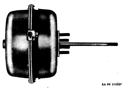
Figure 106—D-64 Power Chamber
