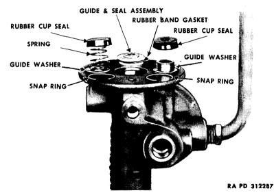
Figure 56—Seal Assembly
