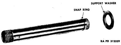
Figure 98—Snap Ring and Support Washer
