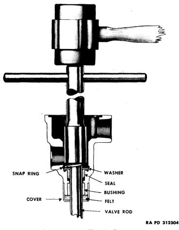
Figure 73—Installing Seal
