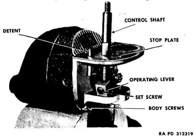
Figure 88—Stop Plate Washer Assembly
