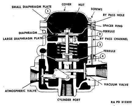
Figure 91—Sectional View of PC Conversion Valve
