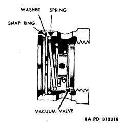
Figure 87—Sectional View of Vacuum Valve Assembly
