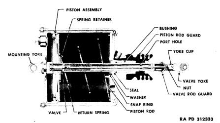
Figure 102—Sectional View of Slide-type Valve Reactionary Internal Valve Power Unit
