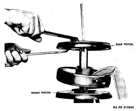
Figure 11—Removing Rear Piston
