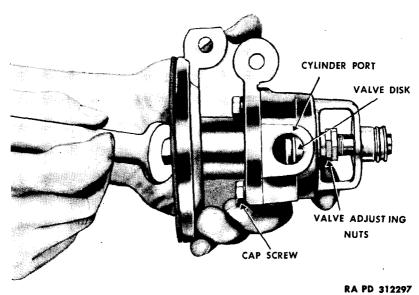
Figure 66—Adjusting Valve Disks
