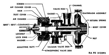
Figure 61—Cross-section of RXL Valve
