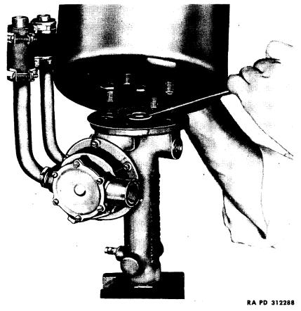
Figure 57—Installing Seal Assembly
