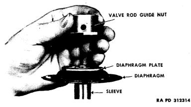
Figure 83—Diaphragm Assembly
