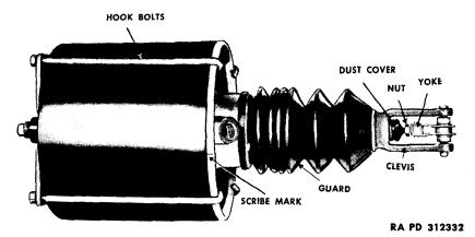
Figure 101—Slide-type Valve Reactionary Internal Valve Power Unit
